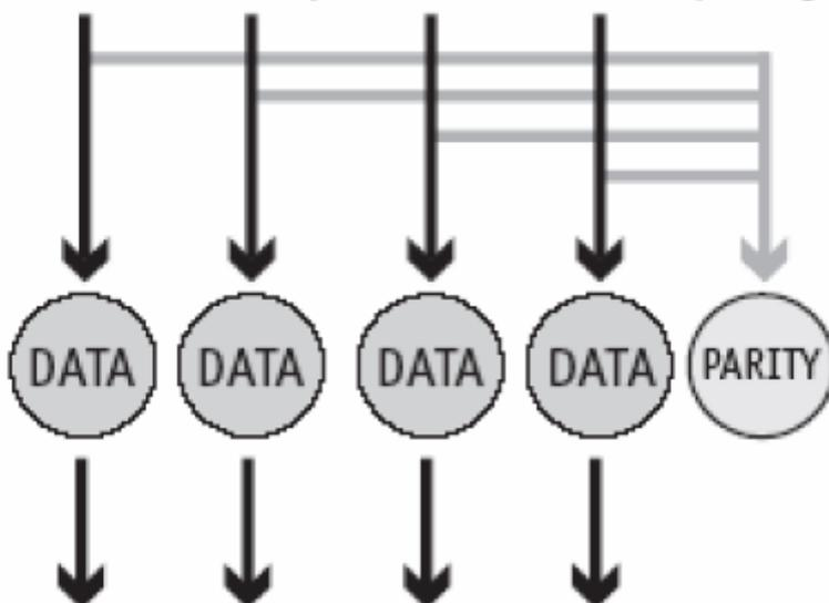
Reads can occur simultaneously on every data drive.
